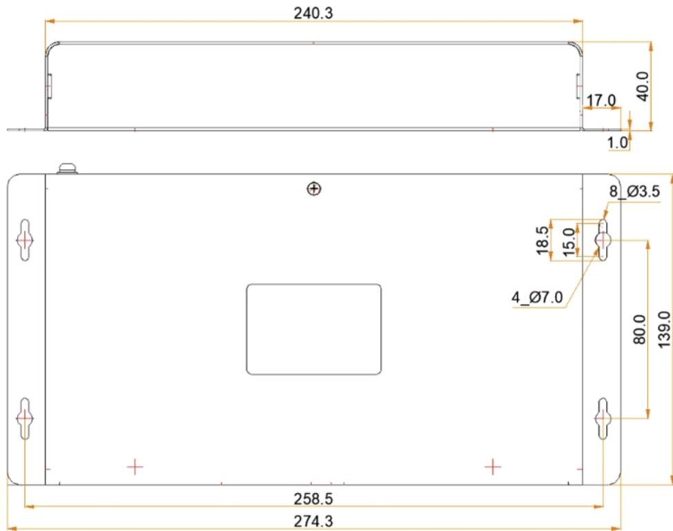
Tolerance:  $\pm 0.3$  Unit: mm
